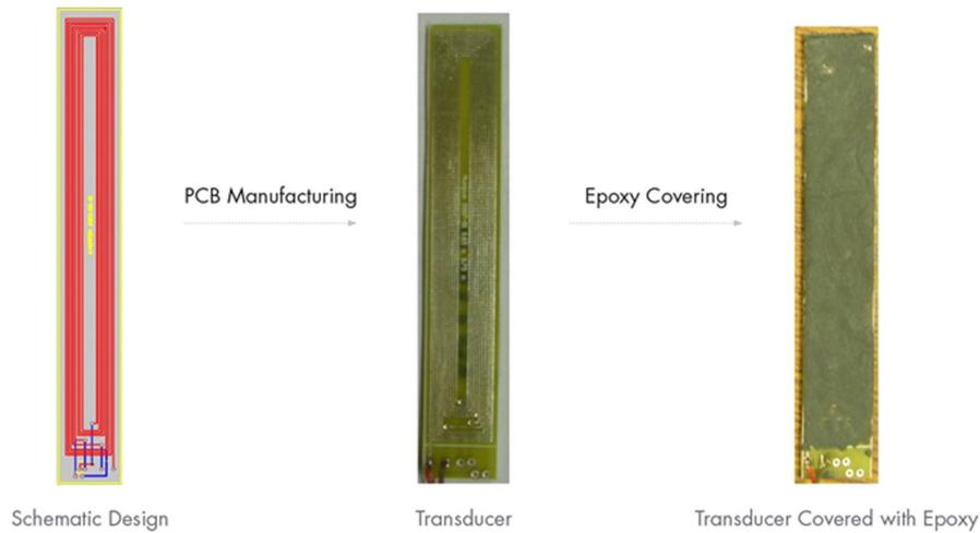
**Fig. 10** Draw-in sensor transducers design and development
