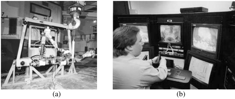
Fig. 1. Argonne's Dual Arm Work Platform consisting of (a) remote robot and cameras, and (b) local user interface
