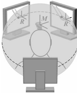
Fig. 9. Method of placing displays on sphere around the user
