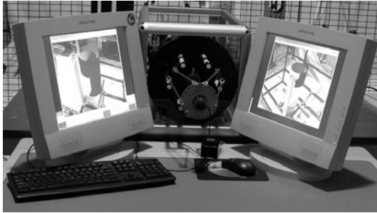
Fig. 11. Mentally efficient interface for Northwestern-Argonne teleoperation
