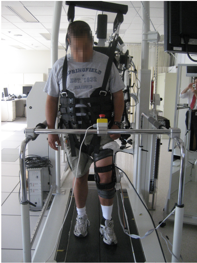
Fig. 5. Experimental setup where subject wears harness to protect from falls. Cables leading to device are for Bowden actuation and sensors, whose weight is partially supported at the bar.
