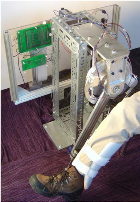
Fig. 3. 1-DOF exoskeleton for assisting knee-joint motion.
