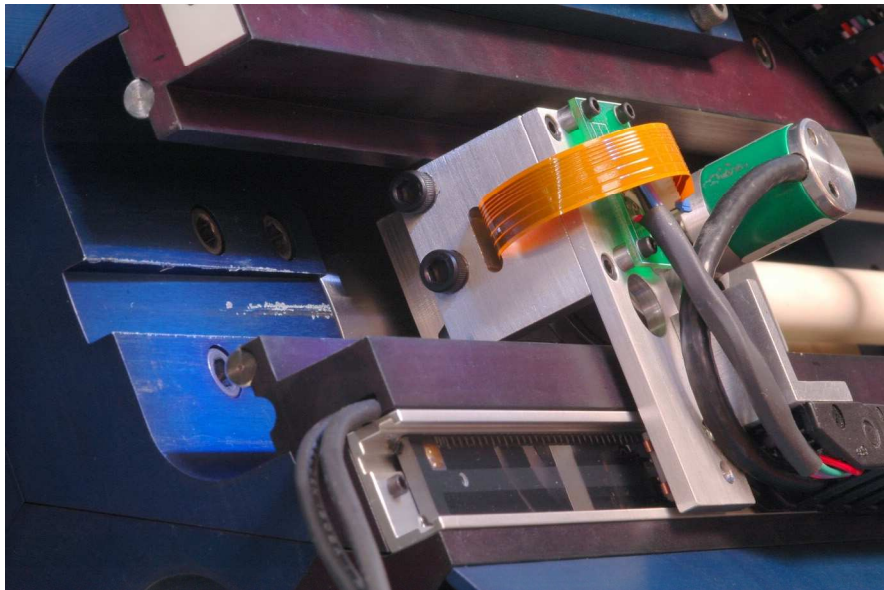
Figure A.11. Ramp for generating preload during insertion of carriage.
