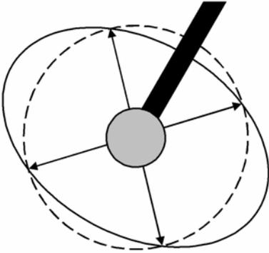
Fig. 6 The intersection of the inertia ellipse of the cobot with the inertia ellipse of a point mass (i.e., a circle) can be used to determine the directions of motion in which the cobot will feel like the point mass. These directions are indicated by the arrows. Note that the cobot cannot emulate masses that are too large (small inertia circles) or too small (large inertia circles).
