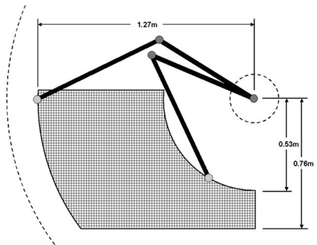
Fig. 10 Using an 80W motor, the UTLA can emulate an 8kg mass over a very large workspace (0.7m<sup>2</sup>). The boundaries of the workspace are physically limited by the table edges on the top, bottom, and right side.
