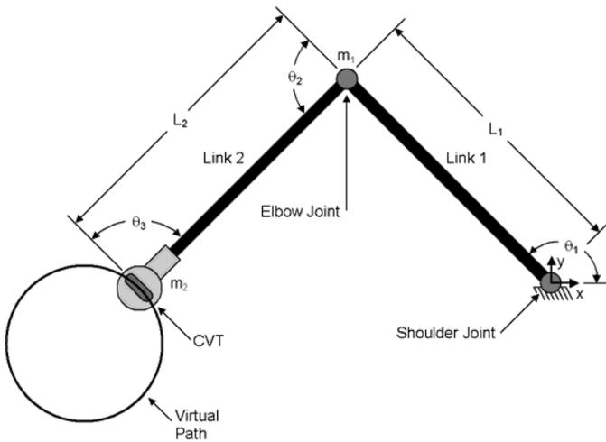
Fig. 2 The motion of the cobot is unintuitive to a user when following certain virtual paths. When the endpoint moves around a circular path, for example, it feels like it is rising and falling. These effects are the result of the apparent inertia varying.
