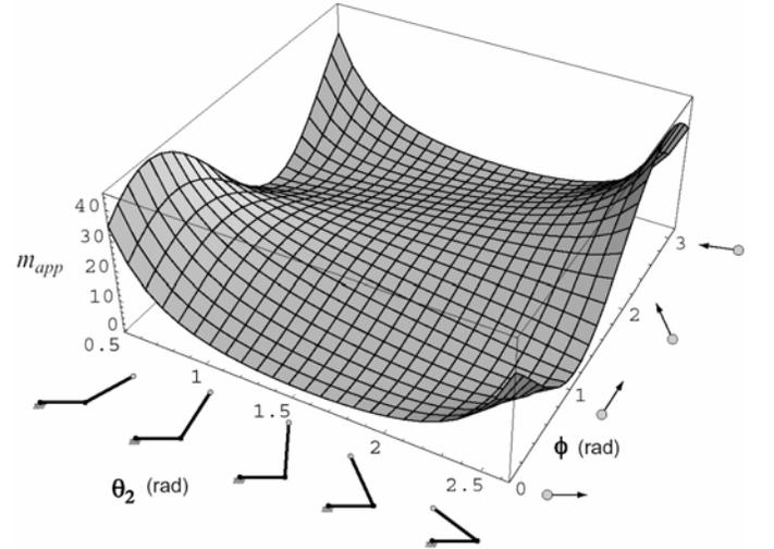
Fig. 4 A three-dimensional plot of the apparent inertia (kg) of the simplified UTLA model is shown as a function of the second joint angle ( $\theta_2$ ) and the angle of motion ( $\phi$ ) of the endpoint. The shoulder joint angle ( $\theta_1$ ) has no affect on the apparent inertia (it only shifts the values), and thus is excluded from consideration.
