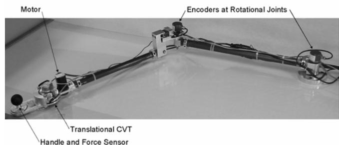
Fig. 1 The unicycle two-link arm (UTLA) cobot is a two-degree-of-freedom haptic device used to display high-quality, software-defined constraints over a workspace large enough for the full motion of a user's arm.
