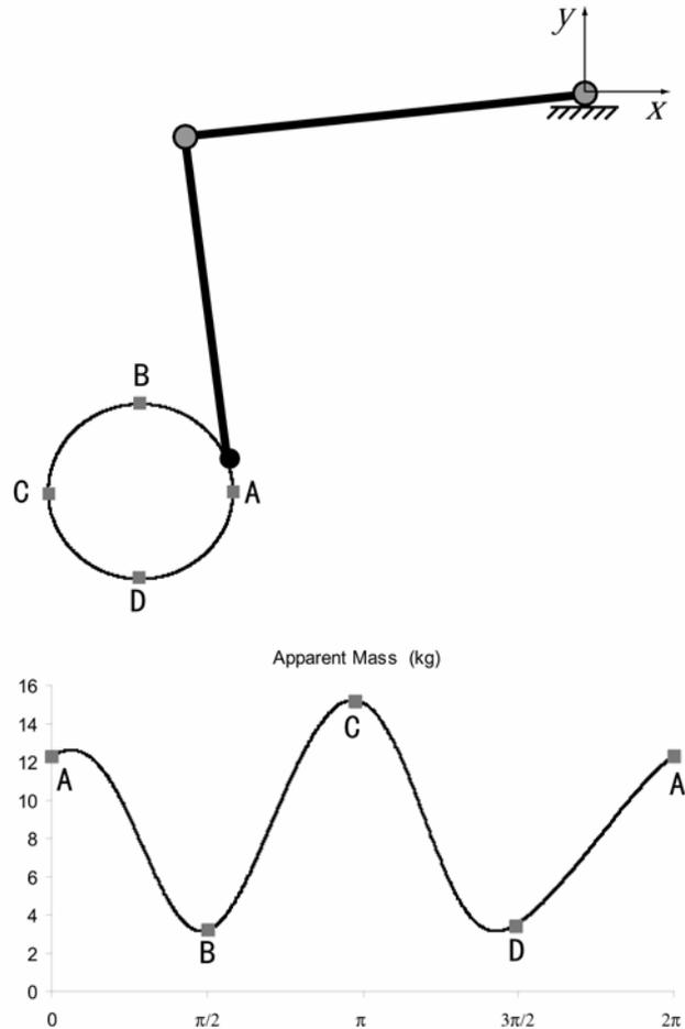
Fig. 3 The apparent inertia of the cobot varies between 3 and 15 kg as a circle is traversed. The radius of the circle shown is 20cm.
