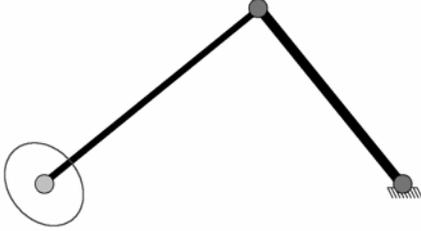
Fig. 5 The long axis of the inertia ellipse corresponds to a direction of low apparent inertia, and the short axis corresponds to a direction of high apparent inertia.
