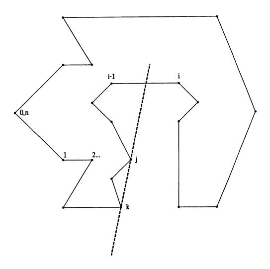
Figure 8: Construction showing the relationship of j, k, and i as used in the convex rope algorithm
