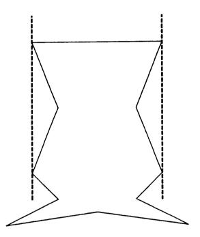
Figure 1: Parallel virtual surfaces (dashed) which form a grasp of the polygon (solid)
