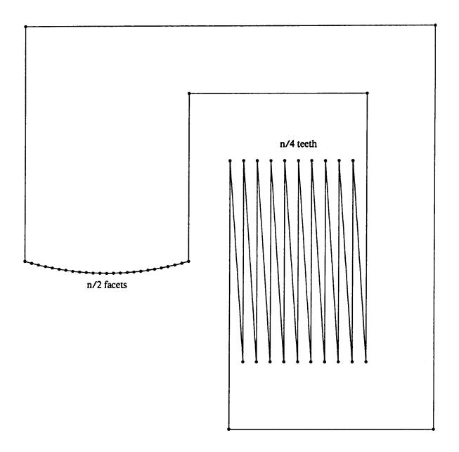
Figure 10: A pathological object which causes the convex rope algorithm to use its worst case number of steps
