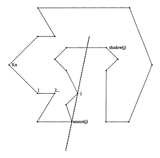
Figure 7: Construction showing the relationship of j, source(j), and shadow(j), as used in the convex rope algorithm
