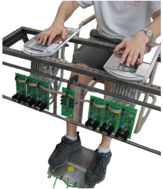
Fig. 3. Participant seated at apparatus. The TPAD assembly for the ring finger of the left hand is lowered in this picture, while the other five assemblies are raised. Both feet are placed on foot switches, but only one switch was used in this experiment.
