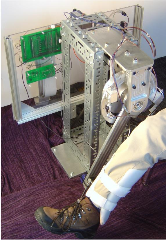
Fig. 3. 1-DOF exoskeleton for assisting knee-joint motion.
