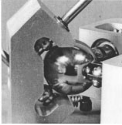
Fig. 9. A prototype of the tetrahedral CVT. The drive rollers are attached to the two shafts on the left (which are perpendicular to each other). The steering rollers are on the right side, and a portion of the gear mechanism which synchronizes the steering rollers is also visible.
