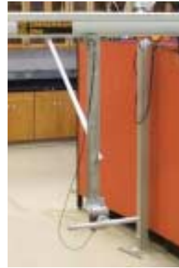
Figure 5: A trolley on an overhead rail system provides a smooth rigid constraint.
