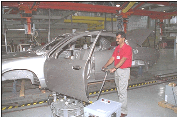
Figure 4: The floor-based cobot door unloader (courtesy of General Motors Corporation)
