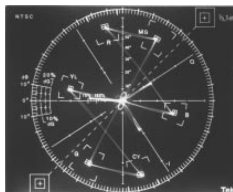
Vector Plot of Standard Color Burst
