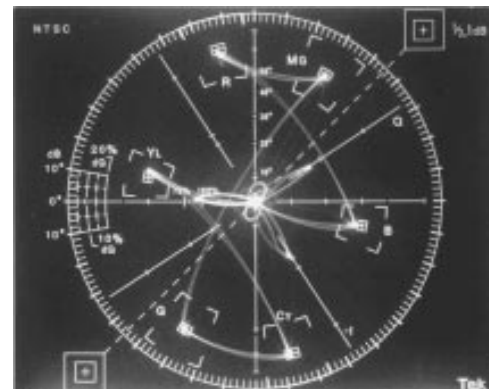
Vector Plot of Standard Color Burst Through 1000 Feet of Twisted-Pair
