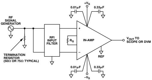
Figure 8. Typical Test Setup for Measuring an In-Amp's RFI Rejection
