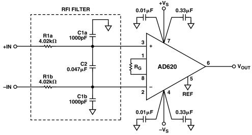
Figure 3. RFI Circuit for AD620 Series In-Amps
