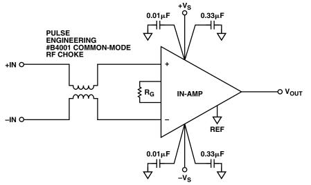
Figure 7. Using a Commercial Common-Mode RF Choke for RFI Suppression
