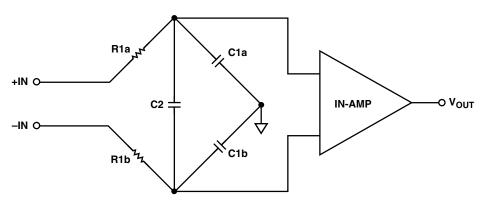
Figure 2. Capacitor C2 Shunts C1a/C1b and Very Effectively Reduces AC CMR Errors Due to Component Mismatching
