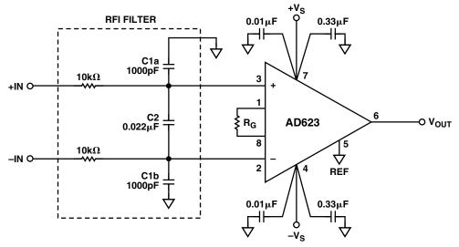
Figure 5. AD623 RFI Suppression Circuit
