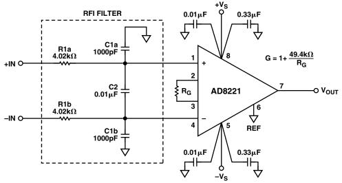
Figure 1. LP Filter Circuit to Prevent RFI Rectification Errors
